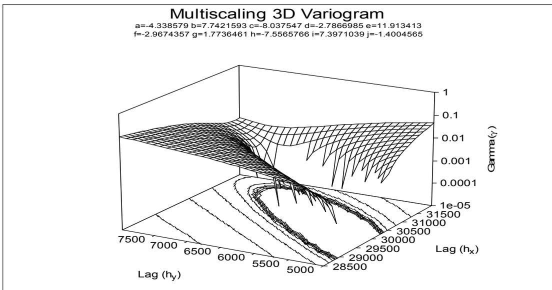
Fig. 2. Multiscaling 3D variogram based on data of Copper-Gold ore deposit "Chelopech". In top of figure the arguments of the approximating function are showed. Wide scale dependence is fixed from a "rounded" part of the function, and small-scale is fixed in bottom the profiles, where the level lines, have merged. Variances in meters is from some hundreds meter for LRD and some meters for SRD-ed.
