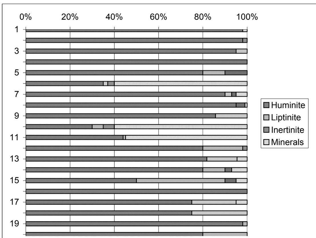
Fig. 1. Distribution of maceral groups and mineral content in the seam profile. Axis X – percentage content of the maceral groups and mineral content. Axis Y – number of samples (20), sampled at 20 cm in the seam profile.
