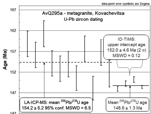
**Fig. 2.** *In situ* LA-ICP-MS  $^{206}\text{Pb}/^{238}\text{U}$  ages for zircons of sample AvQ295a. The TIMS data are shown for comparison.
