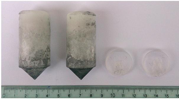
**Fig. 1.** From left to right grown boules and their slices from Sample 1 and Sample 2, respectively
