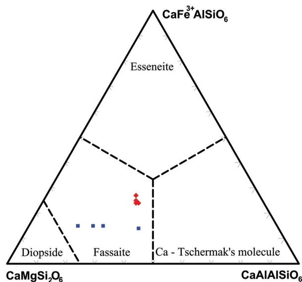
**Fig. 1.** Clinopyroxene compositions in the system CaMgSi<sub>2</sub>O<sub>6</sub>–CaFe<sup>3+</sup>AlSiO<sub>6</sub>–CaAlAlSiO<sub>6</sub> (according to Cosca and Peacor, 1987); blue squares, original bricks; red rhombs, new bricks
