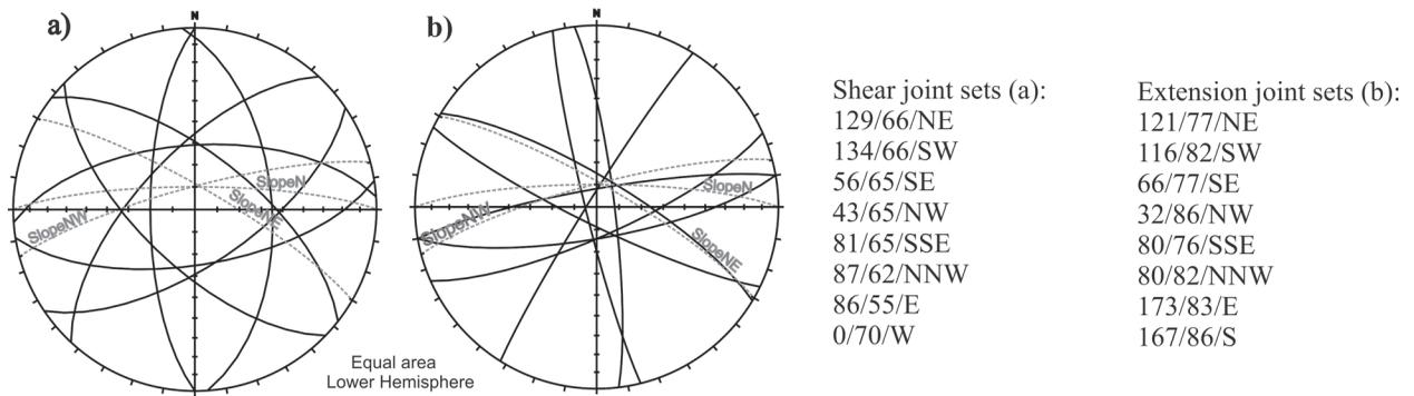
**Fig. 1.** Stereographic plots of joints from the rockfall area: *a*, large circles representing the maximum values in the orientation of shear joints; *b*, extension joints. The dashed large circles represent the orientation of the rock slopes.
