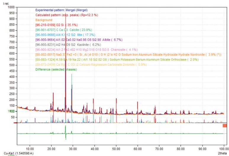
Fig. 1. X-ray diffractogram
