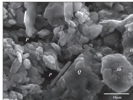
Fig. 2. SEM image of marl of 200 m depth (P-5 BH, Golyamo Peshtene area) – microporosity (P), quartz grains (Q), albit grains (Ab) and Illite (Il) are seen in the marl matrix
