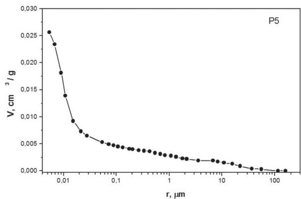
Fig. 3. Pore volume distribution by pore radius
