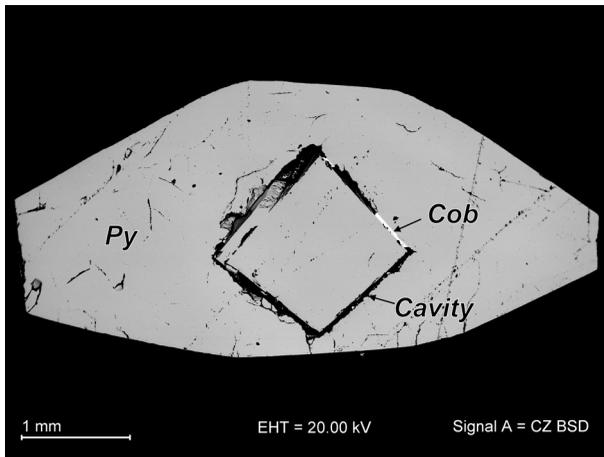
**Fig. 2.** Polished section of composite crystal of pyrite nearly perpendicular to [100] direction; “phantom” is located in the central part of the composite crystal; *Cob*, cobaltite; *Py*, pyrite. BSE image.
