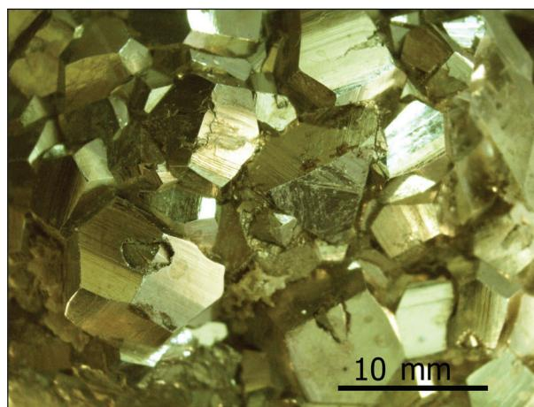
**Fig. 1.** Pyrite druse. Each of pyrite crystals shows signs of dissolution and consists of octahedral {111} “phantom” and rounded external {210}+{211} forms. Optical microscope image.
