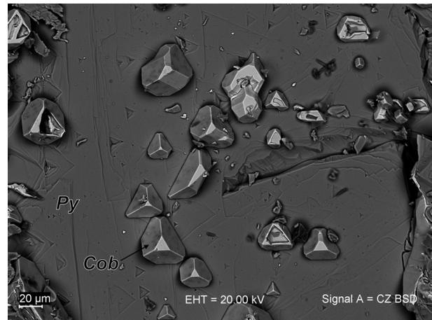
**Fig. 3.** {111} surface of the “phantom” crystal sporadically covered by strongly oriented cobaltite microcrystals; *Cob*, cobaltite; *Py*, pyrite. BSE image.
