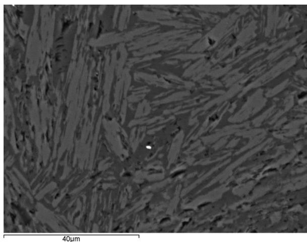
Fig. 1. BSE image of diaspore (dark grey) and corundum (light grey)
