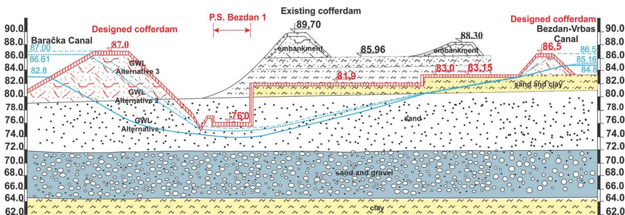
Fig. 1. Lowering of the water table as a result of groundwater control system operation according to the alternative solutions (A<sub>1</sub>, A<sub>2</sub>, A<sub>3</sub>)
