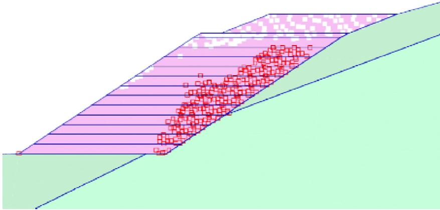
Fig. 13. Plastic points from the finite element analysis
