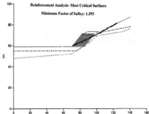
Fig. 6. Initial design of reinforced slope for 1.5:1 slope
