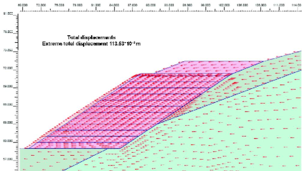
Fig. 11. Extreme total displacement vectors in the reinforced slope mass
