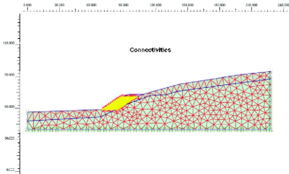
Fig. 10. Finite element mesh for the reinforced slope
