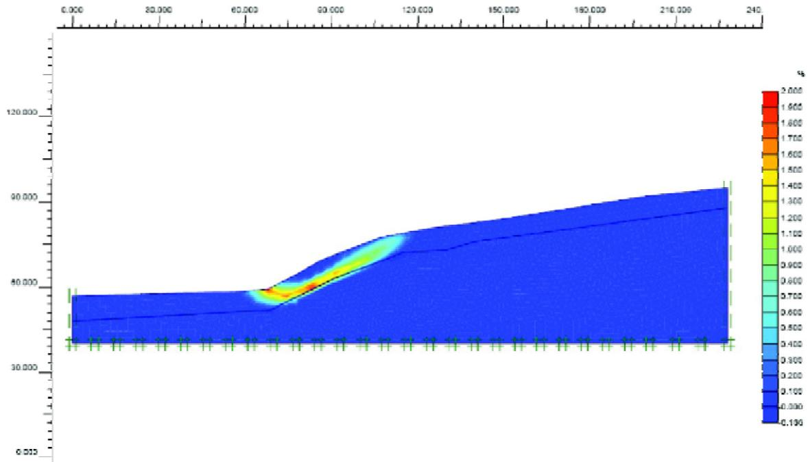
Fig. 15. Shear strains within the unreinforced embankment revealing circular failure surface
