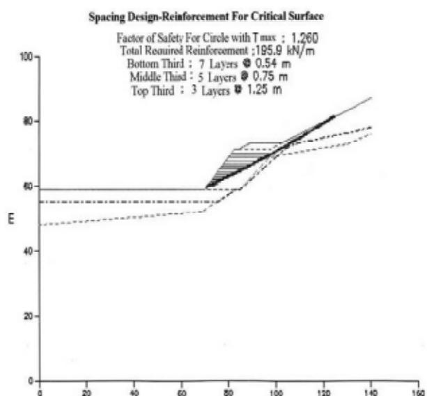
Fig. 7. Reinforced Soil Slopes (RSS) design for 1.5: 1 slope
