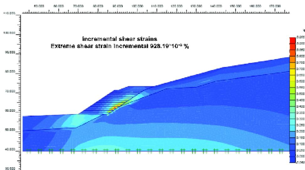
Fig. 12. Incremental shear strains within the reinforced mass
