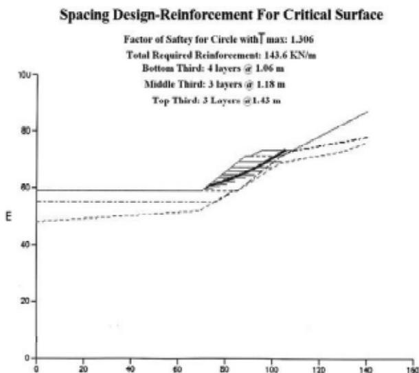
Fig. 9. RSS design for 1:1 slope
