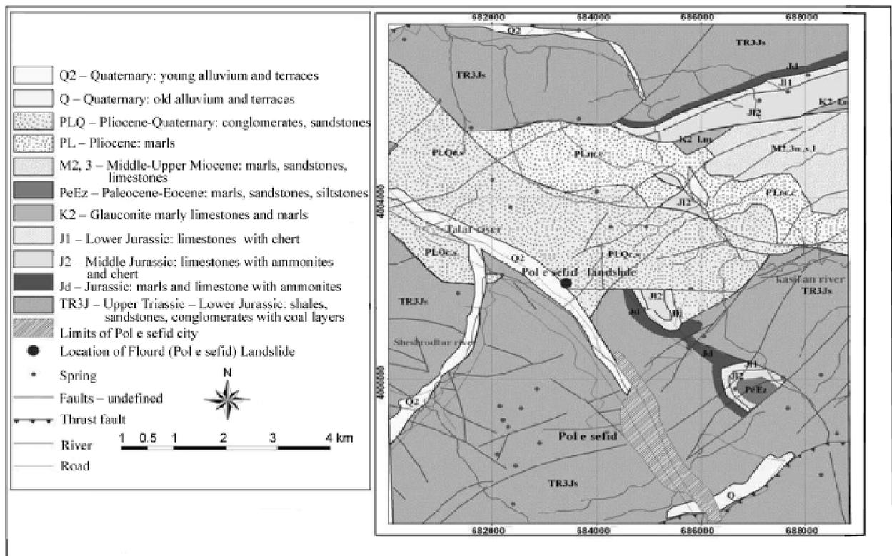
Fig. 2. Geological map of Pol e sefid area with location of Flourd landslide (After Pazoki et al., 2003).
