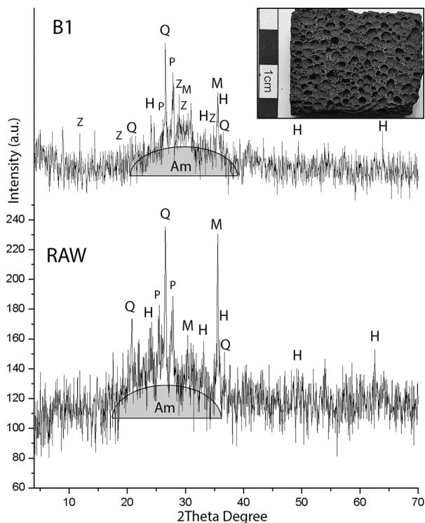
Fig. 1. Powder XRD results for the fly ash (raw) and the prepared geopolymer (B1); Q, quartz; M, magnetite; H, hematite, P, plagioclase, Z,  $\text{Na}_8\text{KS}_9\text{O}_{18}(\text{OH})_9 \cdot 19\text{H}_2\text{O}$ . Right corner – image of piece from sample LB1.
