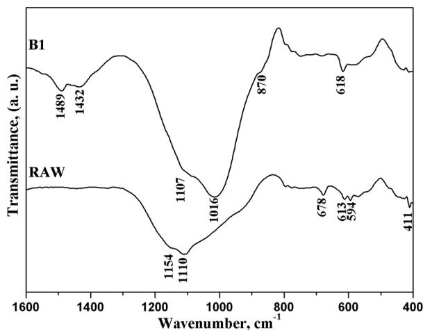
Fig. 2. FTIR spectra of the raw fly ash and geopolymer B1
