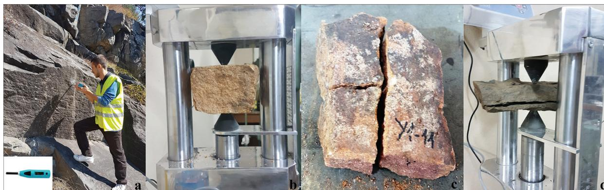
Fig. 1. Implementation of RHM and PLT: a, RHM application on site; b, PLT of sandstone; c, sandstone after failure; d, argillite after failure
