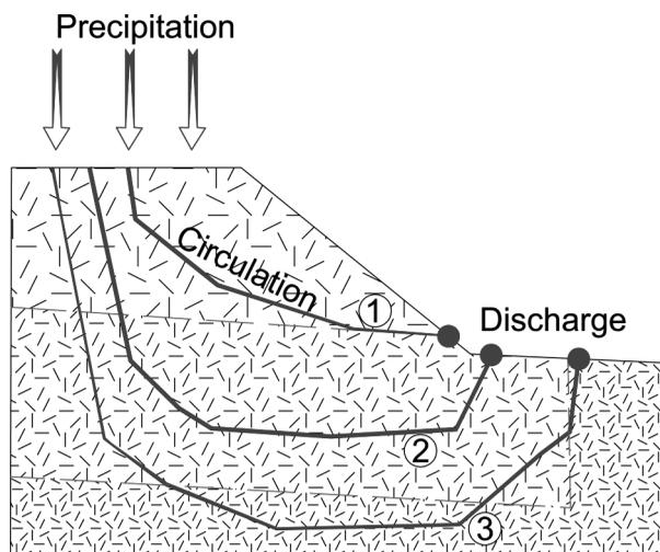
**Fig. 2.** Conceptual model of draining and circulation of the karstic springs: 1, gravitational circulation; 2, siphonal circulation/rapid water exchange; 3, siphonal circulation/slow water exchange (after Vasić et al., 2013, modified)
