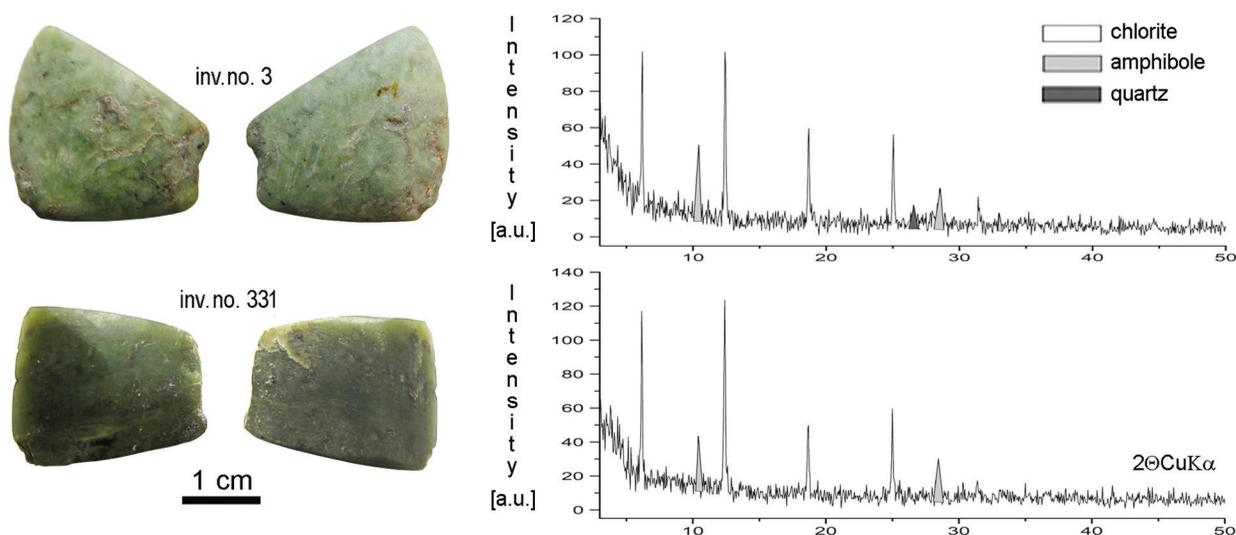
Fig. 1. The studied stone tools seen from the two larger sides (left) and the respective X-ray powder diffraction patterns (right)
