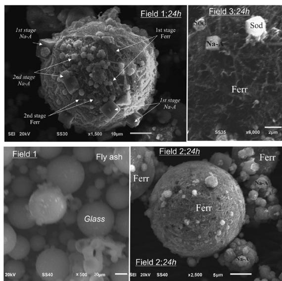
**Fig. 1.** PXRD patterns and SEM micrographs of the products obtained from the low-temperature (70 °C) hydrothermal treatment of fly ash with 1.25M NaAl(OH)<sub>4</sub>
