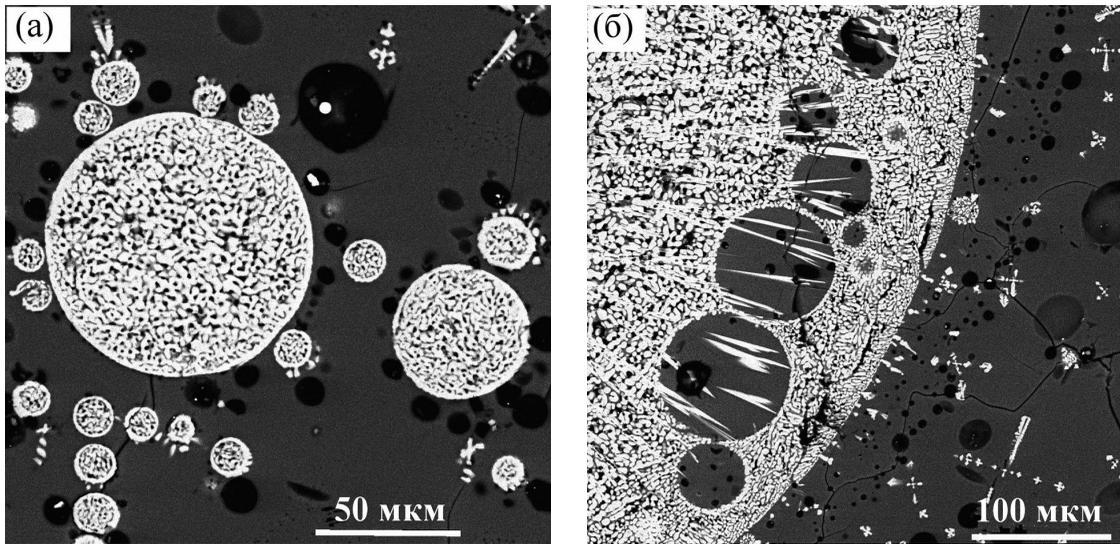
**Fig. 1.** (a, b) Liquid immiscibility between silicate (dark) and fluoride-Ca (light) melts, obtained at T 1250 °C and P 5.5 kbar. BSE image.
