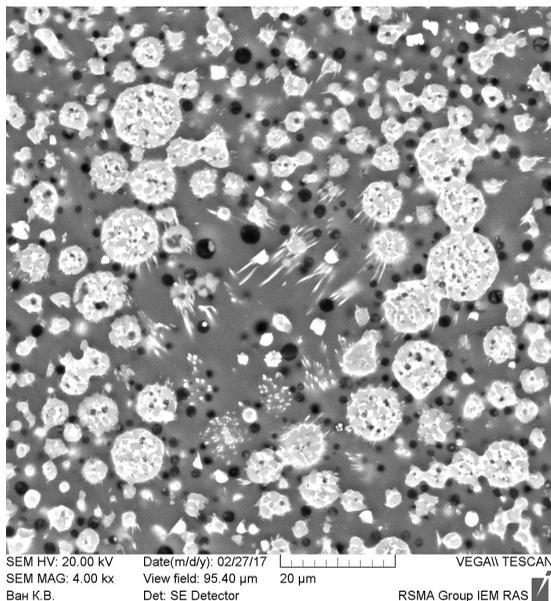
**Fig. 2.** Liquid immiscibility between silicate (dark) and fluoride-Ca (light) melts, obtained during melting of mixtures of trachyrhyolites with minimum and maximum F contents in ratio 1:2 (9.40 wt% F) at T 1250 °C and P 5.5 kbar. BSE image.
