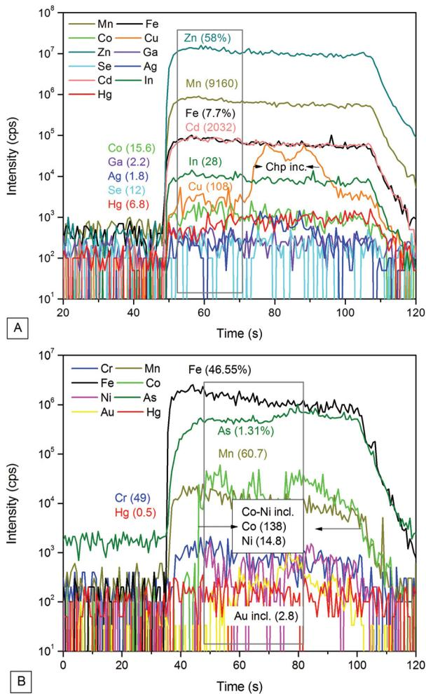
**Fig. 1.** Representative LA-ICP-MS depth spectra of sphalerite (A) and pyrite (B). Numbers in brackets are concentration (in ppm, except otherwise cited). Chp, chalcopyrite; incl., inclusion
