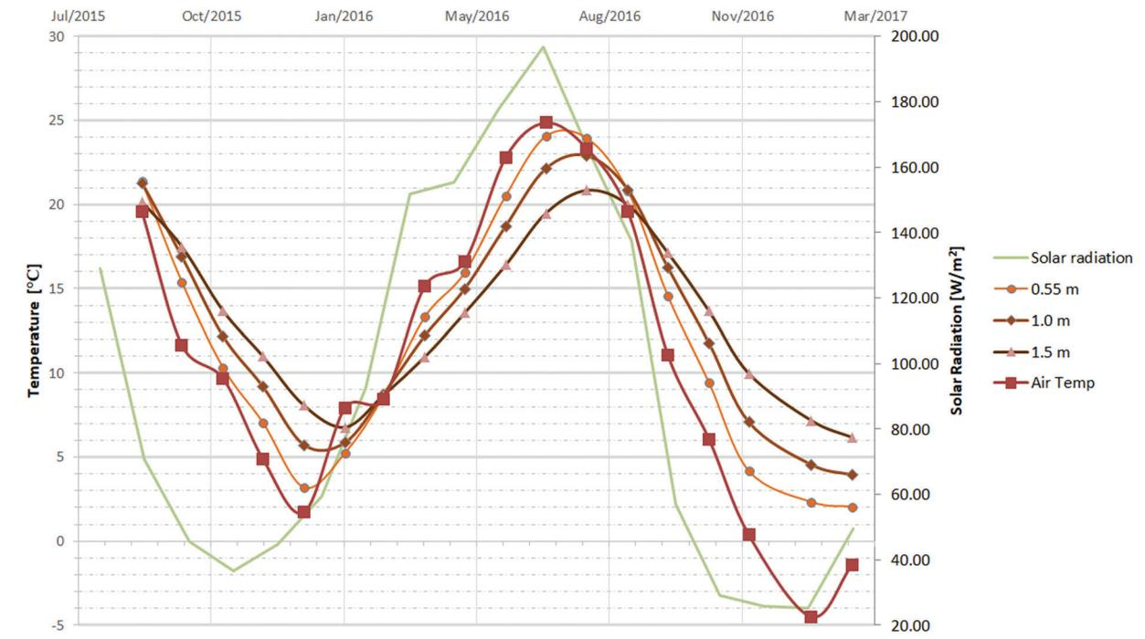
Fig. 1. Monthly variations of the solar radiation, air temperature and soil temperature in the upper part of the loess deposits
