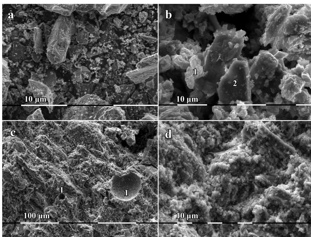
Fig. 1. SEM images of: a, raw fayalite; b, geopolymer cement (Fayalite + SP); c–d, geopolymer GFP250
