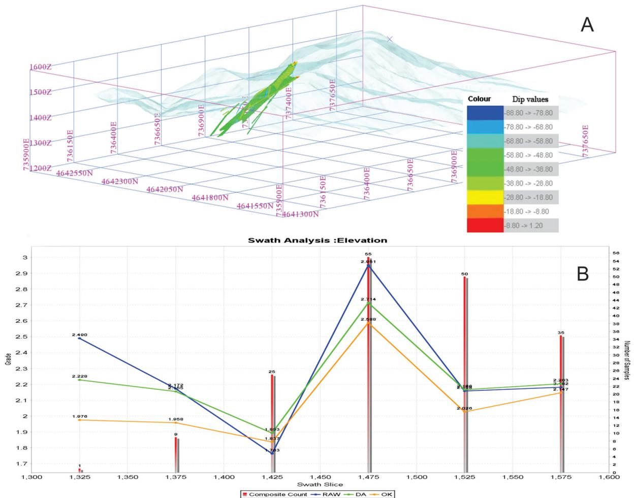
Fig. 1. Block modeling results: A, 3D model of the estimation domains and the local dip angles obtained for each block. The colors assigned to the attribute values of angles are shown in the legend; B, swath plots for sample (raw) data vs Ordinary Kriging (OK) and Dynamic anisotropy (DA) estimates at steps of 50 m in vertical direction.
