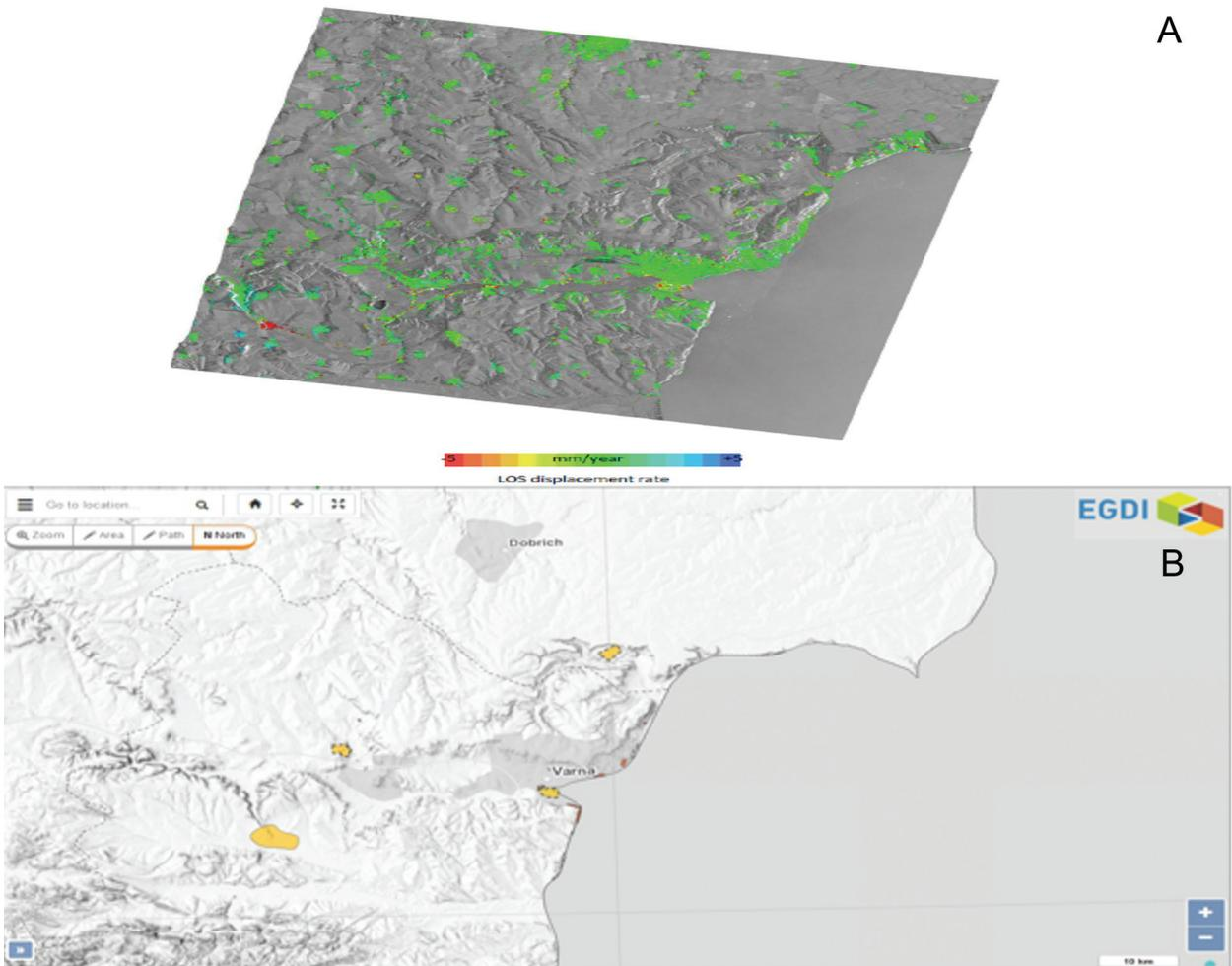
**Fig. 1.** GeoHazard Description for the Varna region. *A*, Varna average line-of-sight displacement map derived using PSI on ASAR data 2003–2009; *B*, Pangeo results for the Varna Region – published on EGDI (European Geological Data Infrastructure) website. Color polygons display types of geological hazards, grey polygons – signal reflection areas.
