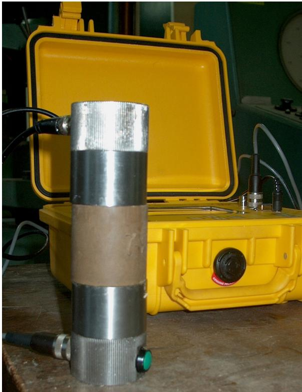
Fig. 1. Ultrasonic testing for determination of the dynamic elastic parameters
