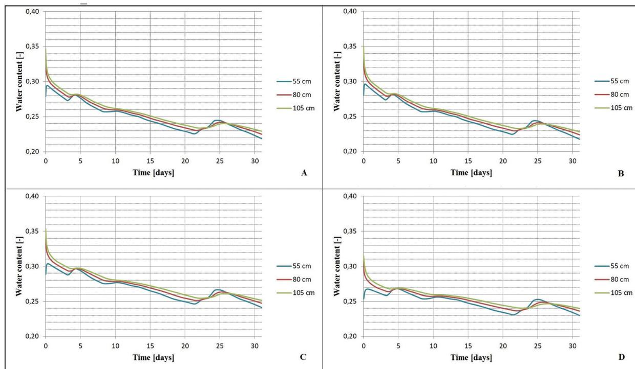
Fig. 1. The obtained moisture content at three depths in the March 2016 period for the investigated case studies
