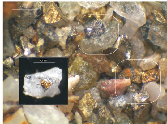
**Fig. 5.** Mineral composition of tailings dam material – main sulfide minerals; intergrowth of sulfides with quartz
