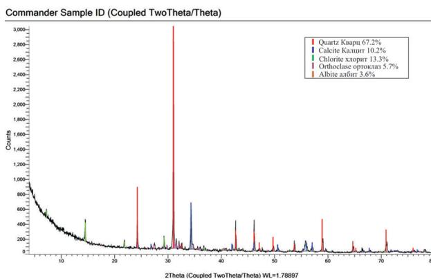
**Fig. 3.** Mineral composition of tailings dam material – main minerals
