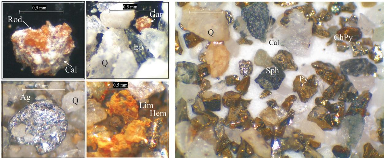
**Fig. 4.** Mineral composition of tailings dam material – rare minerals (Rod, rhodonite; Cal, calcite; Ag, silver; Gar, garnet; Ep, epidote; Q, quartz; Py, pyrite; ChPy, chalcopyrite; Lim, limonite; Hem, hematite)
