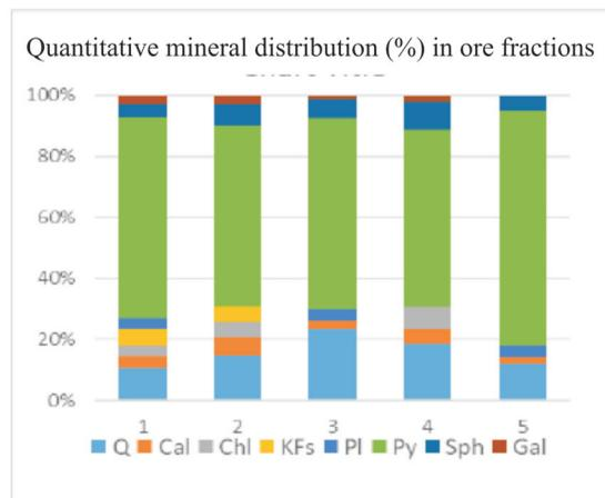
**Fig. 7.** Tailings dam material: “tongues” upstream and stratification of tailings sediments – diagram of quantitative ratio of minerals according to XRD analysis (symbols: Q, quartz; Cal, calcite; Chl, chlorite; KFs, potassium feldspar; Pl, plagioclase; Py, pyrite; Sph, sphalerite; Gal, galena)
