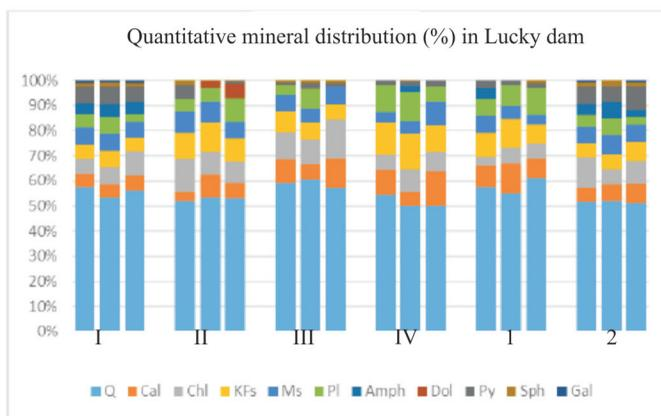
**Fig. 6.** Tailings dam material: average shaft samples – diagram of quantitative ratio of minerals according to XRD analysis (symbols: Q, quartz; Cal, calcite; Chl, chlorite; Amph, amphibole; KFs, potassium feldspar; Ms, muscovite; Pl, plagioclase; Dol, dolomite; Py, pyrite; Sph, sphalerite; Gal, galena)
