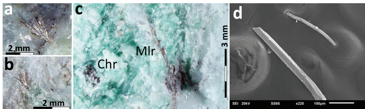
Fig. 1. a , millerite radial fan of acicular crystals within dolomite (Mogilata deposit); b , millerite within dolomite (Krushev Dol deposit); c , millerite and chromite within green mariposite (Krushev Dol deposit); d , SEM microphotographs of millerite crystals (Krushev Dol deposit)
